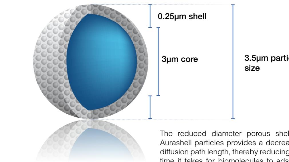
The reduced diameter porous shell of Aurashell particles provides a decreased diffusion path length, thereby reducing the time it takes for biomolecules to adsorb/desorbs in to and out of the particles
