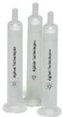
SPE SPE C18 cartridges, A5320320
